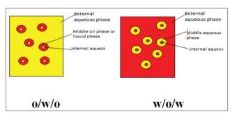
**Figure 2:** Oil-in-water-in-oil and water-in-oil-in-water type of emulsion
