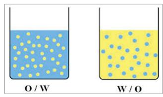
Figure 1: Oil/water and water/oil type emulsion
