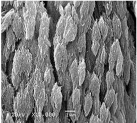
Fig 1: Electronic micrography 10000 magnification of Bone mineral.
