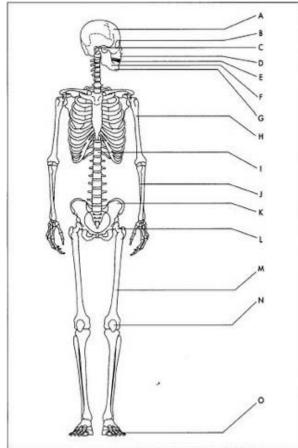
Fig 2: The bioceramic applications. A. Cranial repair. B. Eye lens. C. Ear implants. D. Facial reconstruction. E. Dental implants. F. Jaw augmentation. G. Periodontal pockets. H. Percutaneous devices. 1. Spinal surgery. J. Iliac crest repair. K. Space fillers. L Orthopedic support purposes. M. Orthopedic fillers N. Artificial tendons. O. Joints.<sup>[13]</sup>
