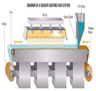
Figure 4: Solvent casting technique
